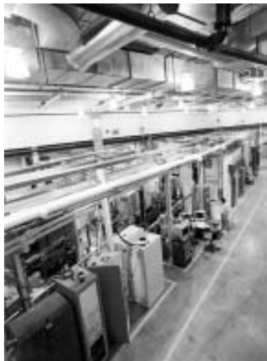
An insertion device beamline on the Advanced Photon Source (APS) experiment hall floor. Photograph courtesy APS at Argonne National Laboratory.
