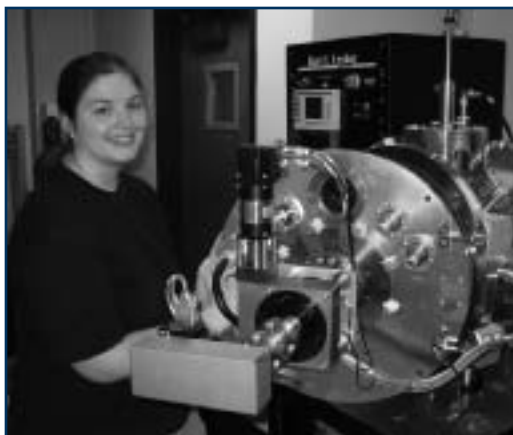
Erin McLellan, a graduate student in the laboratories of Richard Van Duyne and Kenneth Spears, is pictured with an electron beam deposition system used to deposit metal onto prepared surfaces to create nanoparticle arrays. Photograph by Anthony F. Abbinanti.
