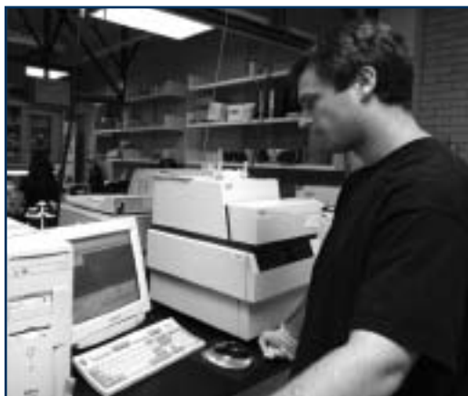
Tom Chiesl is in Annelise Barron’s laboratory. He is pictured running a capillary electrophoresis experiment to measure the amount of protein adsorption onto copolymer matrices. Photograph courtesy of Tom Chiesl.
