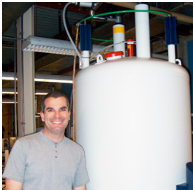
Andrew Ott stands with Northwestern's newest High-Resolution Nuclear Magnetic Resonance spectrometer system, the Bruker 600 MHz Avance III NMR. Photograph by Amanda Morris
